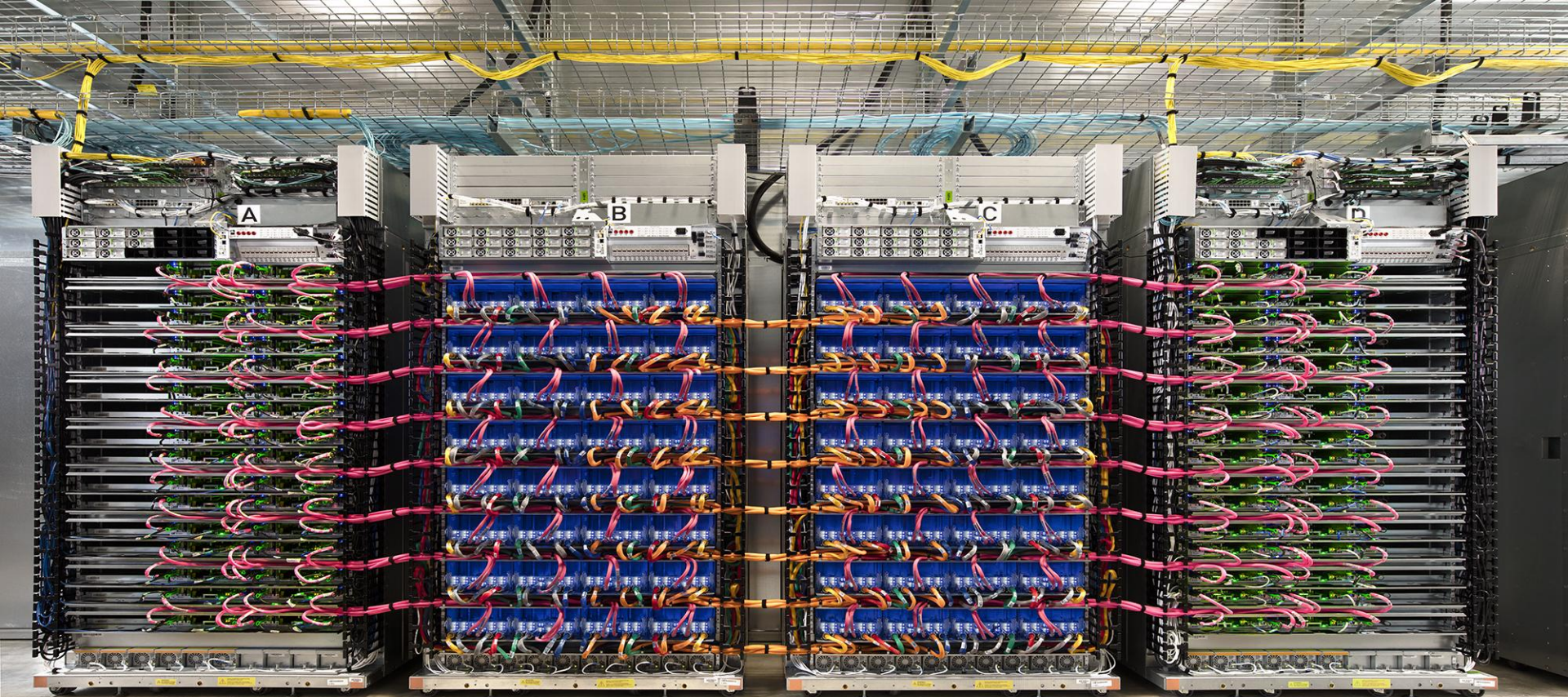
TPU Pod 64 2nd-gen TPUs 11.5 petaflops 4 terabytes of HBM memory
